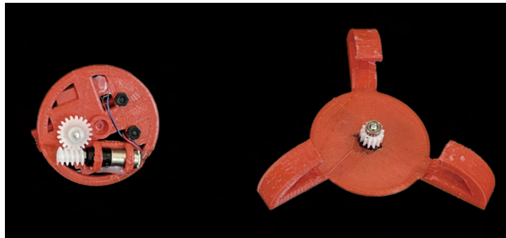
Fig. 8. The turntable mechanism. When the robot makes contact with the copper pads on top and sends a signal through the motor driver, the rotor rotates around the base, which also rotates the robot.
