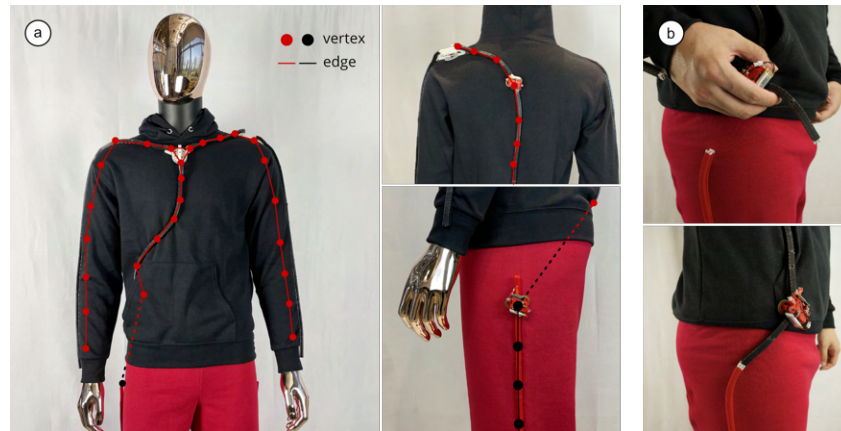
Fig. 9. a) Using a track system on the clothing allows us to project the 3D terrain onto a 2D graph structure to simplify localization. Dotted line indicates temporary magnetic connection. b) The user magnetically connects the tracks to allow the robot to move between upper body and lower body.
