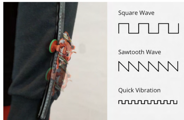
Fig. 10. The different forms of vibration patterns that Calico uses to communicate with the user.
