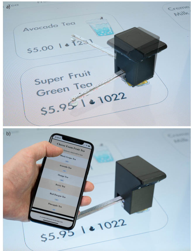
Figure 1: Toucha11y overview. a) The Toucha11y bot can be placed on top of an inaccessible touchscreen kiosk to activate its interface. b) A blind user can access and use the kiosk from their personal smartphone.
